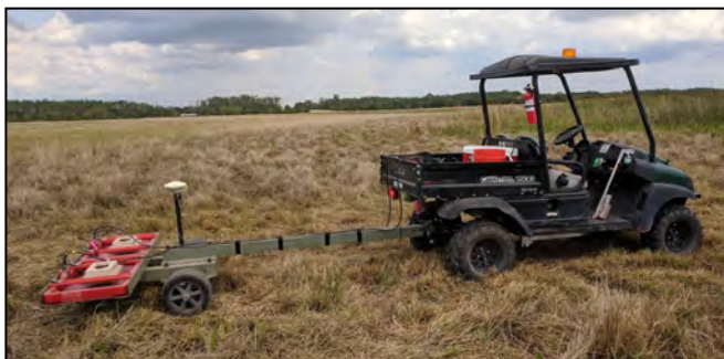
USAE's custom designed EM61 towed array is customizable for 1 to 3 coil array. Left – Two EM Coil configuration. Right – Three EM Coil configuration
