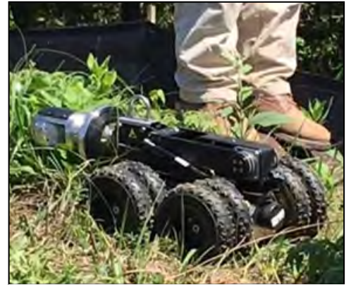
USAE's Pearpoint flexitrax 350 robot being prepared to visually inspect a section of 36" diameter pipe
