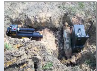
X-Ray Technology In-Field Munitions Identification Using Radiographic Film or Digital Inspection Systems
