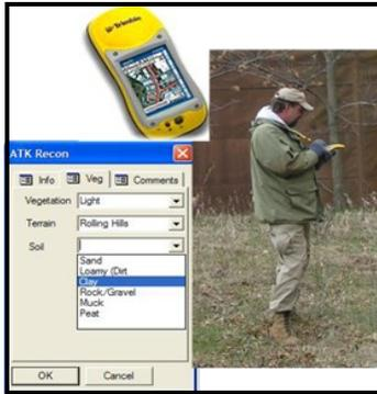
Another good example of USA's proven innovative technology is our GPS interfaced with a PDA, which allows for real-time monitoring of progress in the field. Using the Trimble Geo XT GPS unit and Thales Mobile Mapper CE, we are able to combine sub-meter accurate GPS
