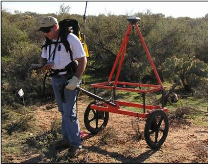
For digital geophysical mapping (DGM), USA and its DGM team members routinely field the latest electromagnetic and magnetometer sensors, includ-
