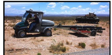
sensor data (VSEMS). USA, working with SAIC, developed, demonstrated, and deploys this system. USA has worked with this system on eight projects. It is exceptionally efficient on large-area surveys where the terrain is vehicular accessible.
