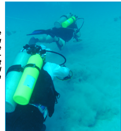
UXO Diver in the rear is conducting QC checks on the UXO Diver swimming a transect during a Remedial Investigation
