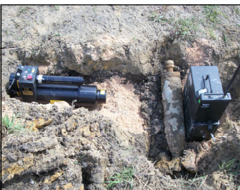
Innovative Technologies Innovative Methods & Advanced Technologies, e.g., X-Ray, (shown) for Effective MEC Field Operations
