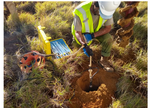
UXO Technician lowering a Bore Hole Gradiometer probe into a geotechnical bore hole, Waikoloa, HI
