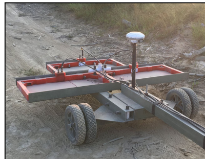
USAE's custom designed EM61 towed array is customizable for 1 to 3 coil array. Left – Two EM Coil configuration. Right – Three EM Coil configuration
