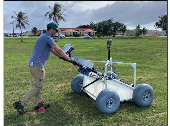
USAE employs White River Technologies' DAGCAP accredited APEX One-Pass AGC sensor, Guam
