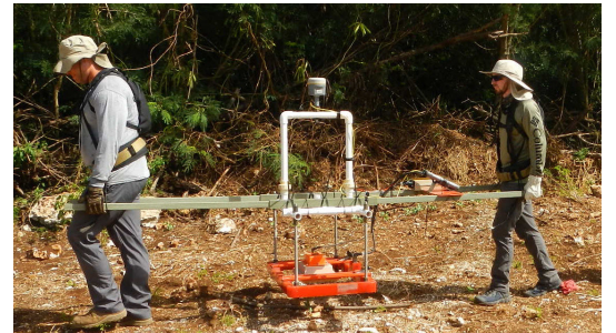
Geonics EM61-MK2A deployed in stretcher mode during DGM survey, Tinian
