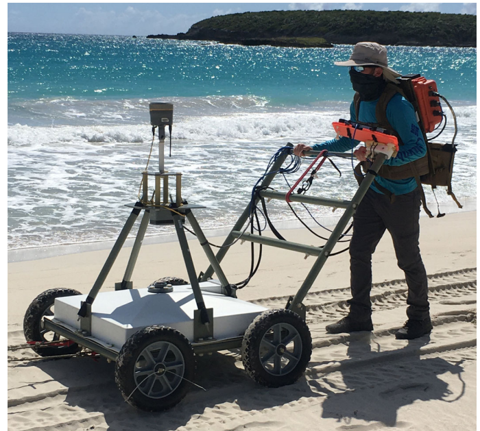
Performing dynamic survey using the Geometrics, Inc., Metal Mapper 2x2 AGC Sensor, Puerto Rico
