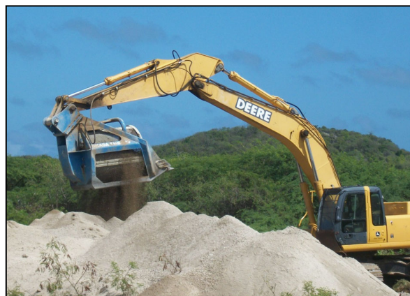
NWDD's Robotic Sifter with Trommel Bucket, Puerto Rico
