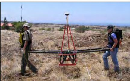
For the EE/CA project at the Waikoloa Maneuver Area, HI, USA evaluated the **multi-gate Electro-magnetic (EM) basalt discrimination developed for the EM63** in
