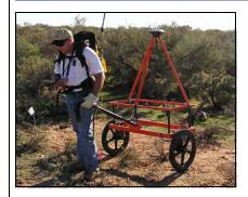
USA provides full digital geophysical mapping (DGM) services. We perform DGM projects, including the support and use of Vehicular Simultaneous Electromagnetic Induction (EMI) and Magnetometer System
