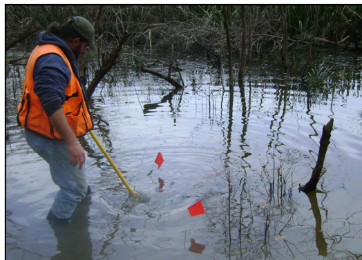
Analog geophysical survey using Schonstedt ferrous metal detector, Camp Maxey, TX
