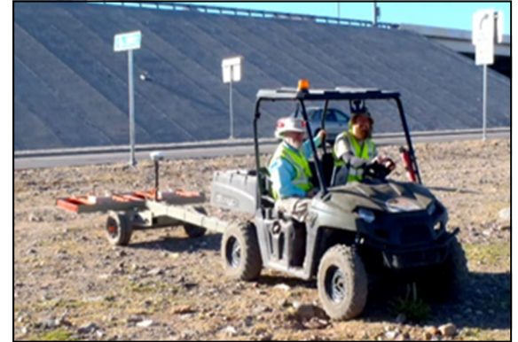
USA's Towed Array performing a dynamic DGM survey at a commercial site in El Paso, TX
