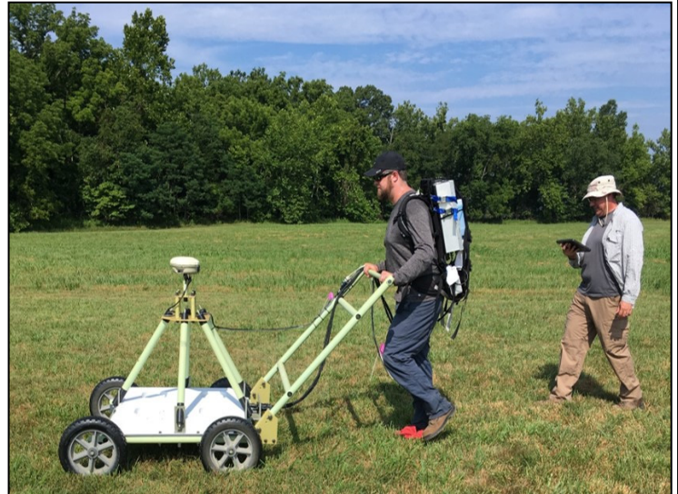
USA Personnel collecting dynamic data with the TEMTADS, Blossom Point, MD
