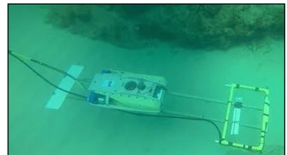
EM61 mounted on ROV during Underwater MEC Survey around environmentally sensitive coral
