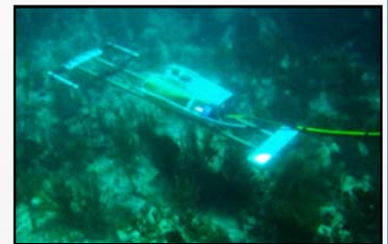
Underwater, an EM61 mounted on an ROV working above environmentally sensitive coral in Culebra, PR (USA)
